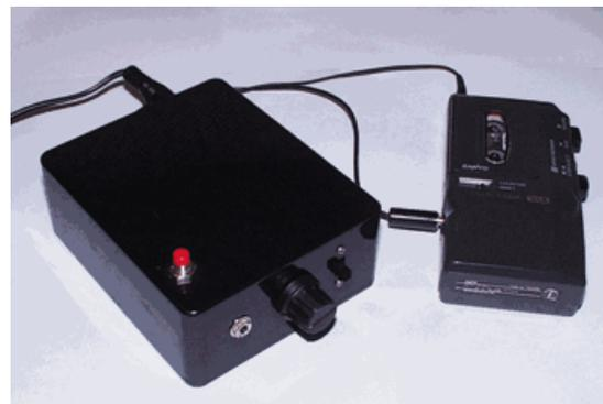
Completed Easy-Typist showing the additional pause-switch button on top of the case.
